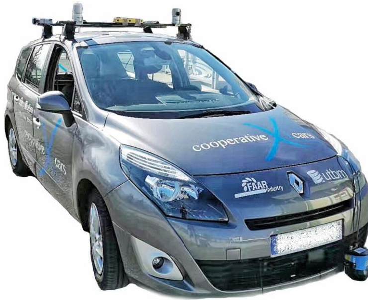
Fig. 1. Automated vehicle equipped with sensors (cameras, lidars, Radar, IMU, GPS, ...) and communications interfaces.
