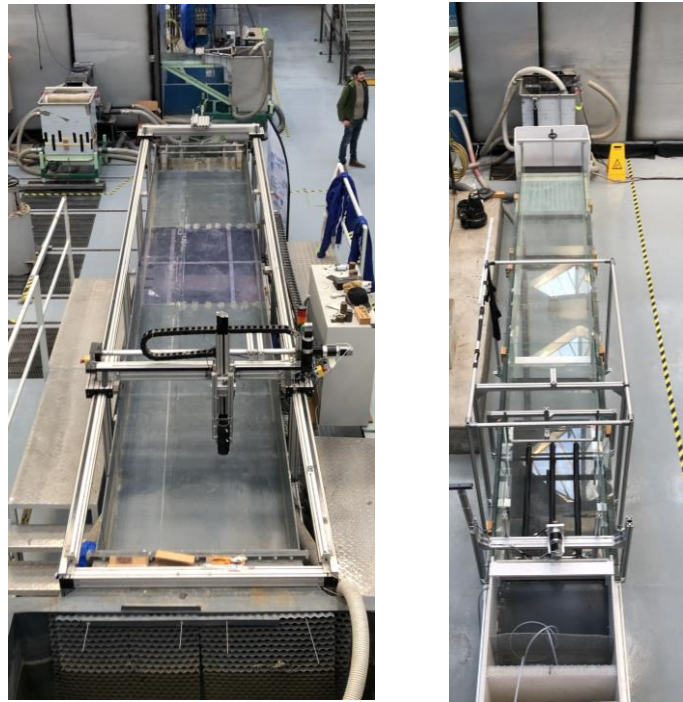
Figure 3: Photographs of the available large scale flume (left) and transparent tilting flume (right)
