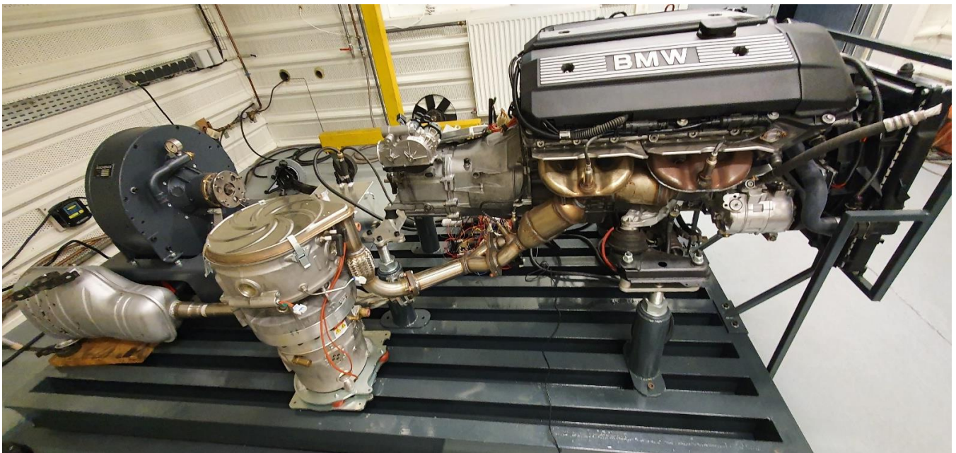
Figure 1: Gasoline internal combustion engine (ICE) coupled via its exhaust gas line to a Stirling engine
