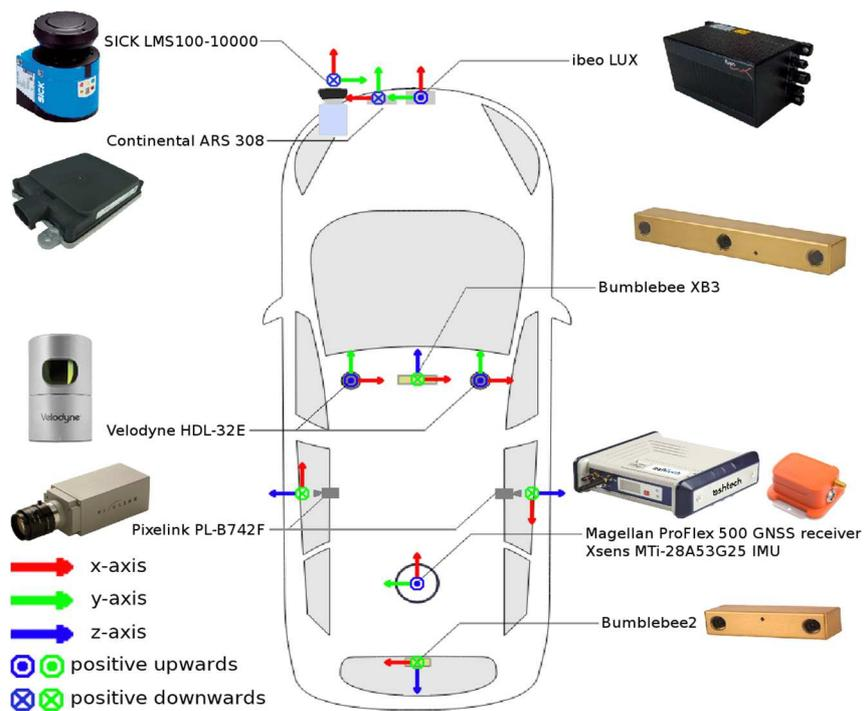
Fig.2. Multi-sensory data acquisition system with heterogeneous sensors.
