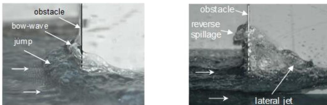
Figure 1: Photographs of the supercritical flow around an obstacle : detached hydraulic jump (left) and wall-jet (right) – from Rivière *et al.*, 2017.
