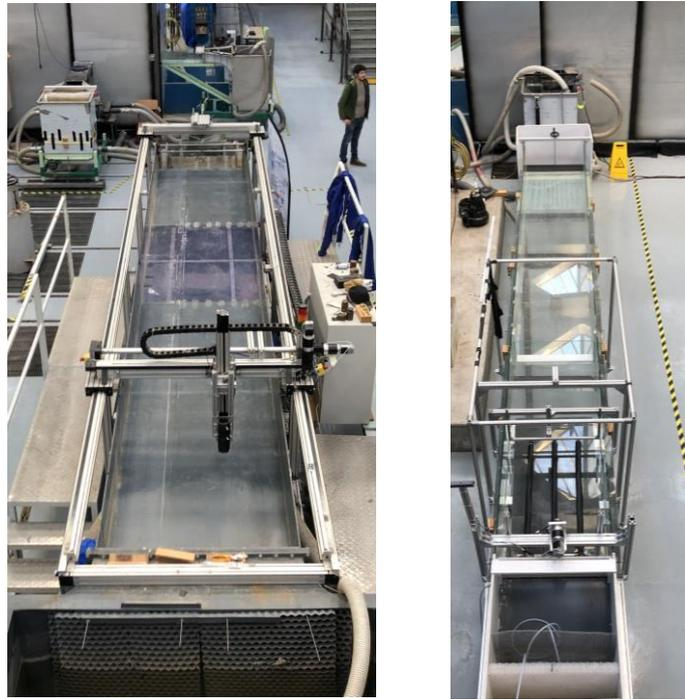
Figure 3: Photographs of the available large scale flume (left) and transparent tilting flume (right)
