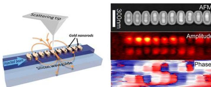
Figure 1: Nearfield optical imaging of a nanostructured integrated photonic waveguide. Left: AFM topography and experimental cartography of the complex optical nearfield [4].
