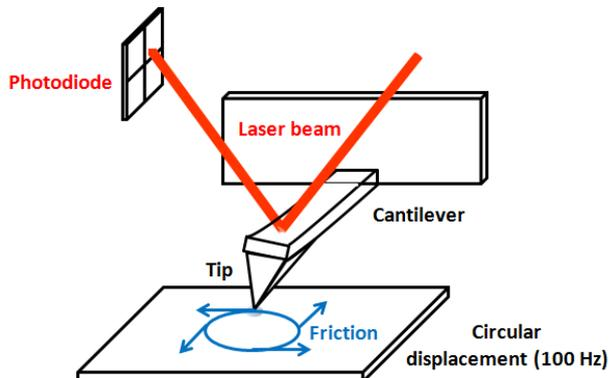
**Fig. 1: Principle of the AFM circular mode. The tip, attached to a cantilever is in contact with the sample and animated by a circular displacement. Normal and friction forces generate flexion and torsion of the cantilever that are detected by the deviation of the laser beam**
