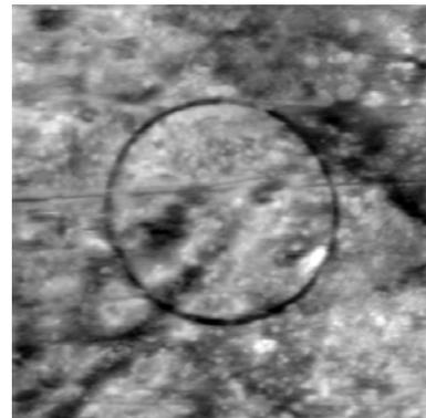
**Fig. 2: Topographic image (x-y scale 5µm, z scale 38nm) of a wear track generated by the AFM in circular mode. The wear track is well defined and the wear volume could be easily computed**
