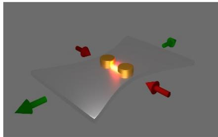
**Figure 3:** Description of the optical measurements with applied strains to the elastomeric substrate in order to investigate variations in the plasmonic coupling.
