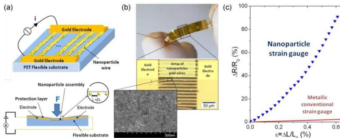
Figure 1: (a) Schematic diagram of a resistive nanoparticle strain gauge, (b) photograph of a strain gauge made of 14 nm gold nanoparticles (top) - image by optical microscopy the active area of the gauge (middle) and image by scanning electron microscopy of the arrangement of nanoparticles (bottom). (c) Relative change of resistance of the strain gauge shown in (b) as a function of strain (the red curve represents the typical response of a conventional metal gauge)
