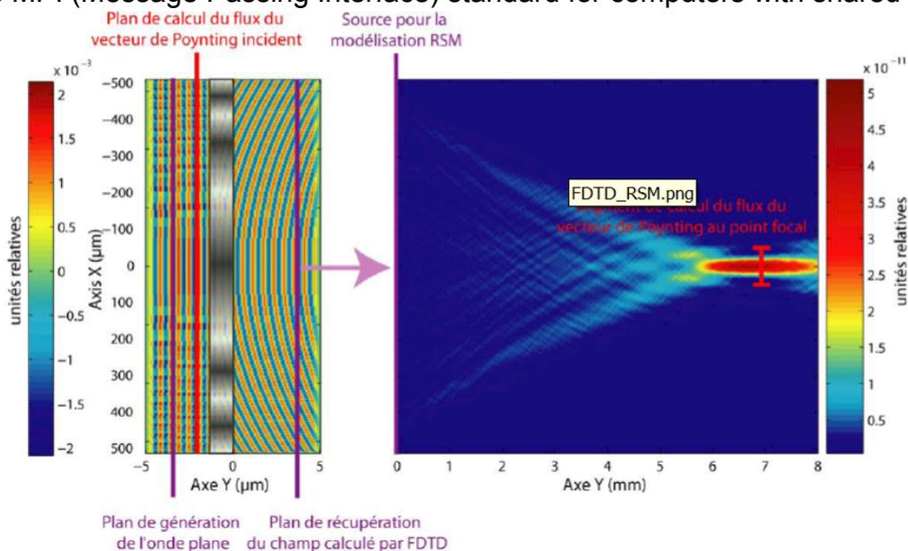
Figure 2: FDTD/RSM combining to compute a Fresnel Lens using the effective medium theory.
