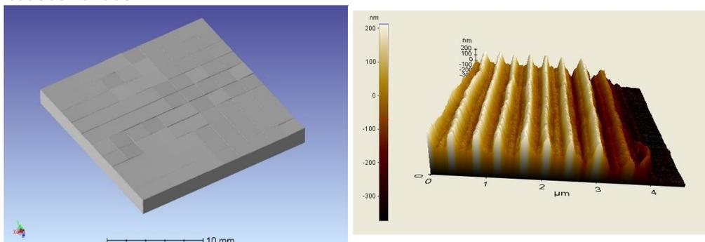
Figure 1 : (Left) Example of the faceted structure designed with Zemax [2]. (Right) Example of a effective medium structure realized by a sub-wavelength grating and measured by AFM. This structure was realized in a previous PhD work in Strasbourg University [4]. A facet structure can be replaced by this type of effective medium.
